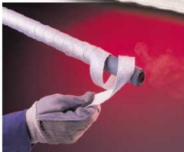
Above, Pipe Wrap (adhesive tape): Pipes can be wrapped with ceramic tape to protect the pipe itself from failing when exposed to high temperature environments. Similarly, the ceramic wrap can help insulate a pipe carrying high temperature fluids. The low conductivity and electrical insulation offered by our ceramic tapes allow for innovative applications such as a beaded resistance wire, needed in processing petroleum products. The electrical current is protected from shorting to the steel pipe by the Nextel ceramic tape.
